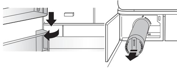
**NOTE:** If the filter is not installed correctly, water may dispense at a lower flow rate and there will be slower ice production. Improper filter installation may also cause the water filter housing to leak.
