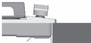
3) Place the hob in the installation opening and push it down so that the hob is resting firmly on the benchtop. Fit the supplied brackets and screws as shown in the illustration right. Tighten the screws to secure the hob to the benchtop.
