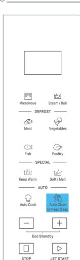
**THIS AUTOMATIC CLEANING** cycle will help you to clean the microwave oven cavity and remove unpleasant odors.
