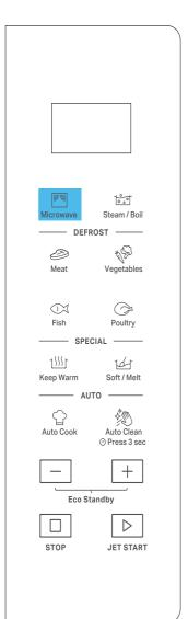
To cook with microwave power individually, press the Micro button repeatly to select a cooking power level, then press +/- button to set a desired cooking time. The longest cooking time is 90 minutes.
