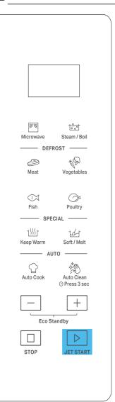
**THIS FEATURE ALLOWS YOU** to start the oven quickly. Press JET START button once, the oven starts work at full power level automatically. During cooking, press JET START to add time. The longest cooking time is 90 minutes.
