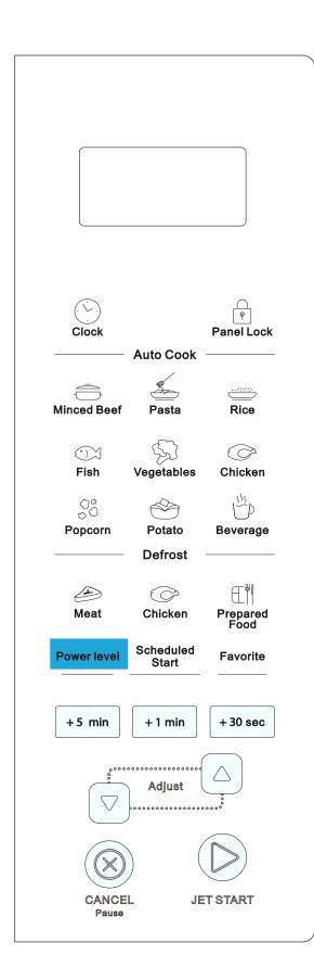
To cook with microwave power individually, press the POWER LEVEL button repeatedly to select a cooking power level, then press the Adjust or Number button to set a desired cooking time. The longest cooking time is 95 minutes.
