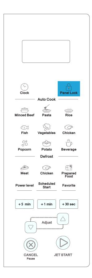
This function is used to prevent unsupervised operation of the oven by children. The indicator Panel Lock will be displayed on the screen, and the oven cannot be operated while the oven is locked and un-activated.
