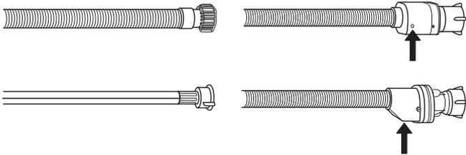
If the inlet hose has a transparent coating, periodically check if the colour intensifies locally. If yes, the hose may have a leak and should be replaced.
